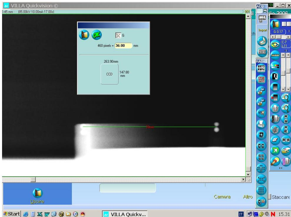
In the measuring window the number of pixel measured is also reported and this measurement is more sensitive, so this is a preferred method. Record the number of pixel (460 in the example).
