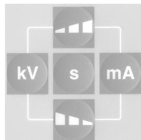
Furthermore there is the possibility to select manually the exposure parameters; in this case select at first the parameter to be changed and secondly, using the increasing and reducing keys, set the required value. The parameters available are: kV and mA.
