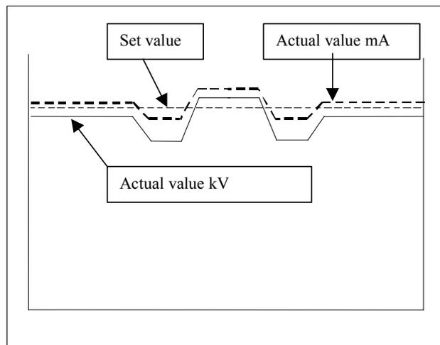
Accuracy declared on the section "Technical data" is referred to the actual value of kV and/or mA. In any case, manufacturer guarantees that the accuracy of loading factors is always compliance with the international standard for safety of medical devices IEC 601-1. Particularly, in accordance with IEC 601-2-7, the maximum deviation (including the correction and instrument's accuracy) is less than or equal to  $\pm 10$  for kV, while for tube current is less than or equal to  $\pm 15\%$ .
