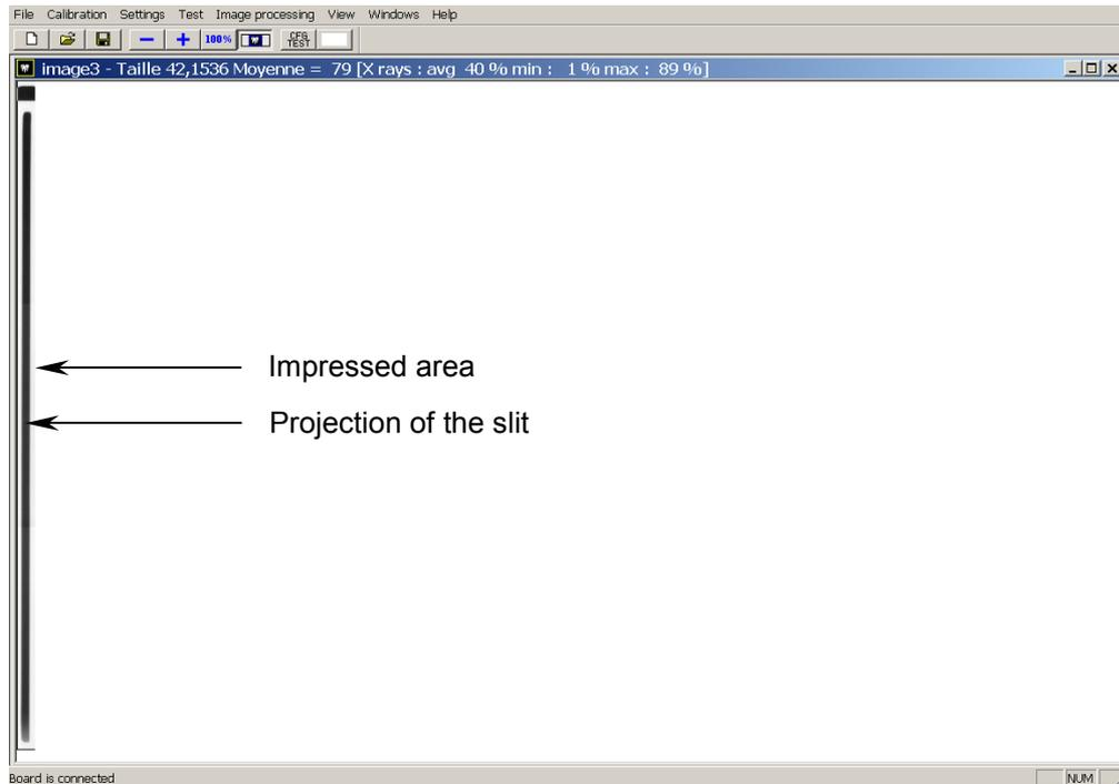
26. In case the alignment is not right refer to paragraph 7.1.3.4 to correct the CEPH sensor setting.
