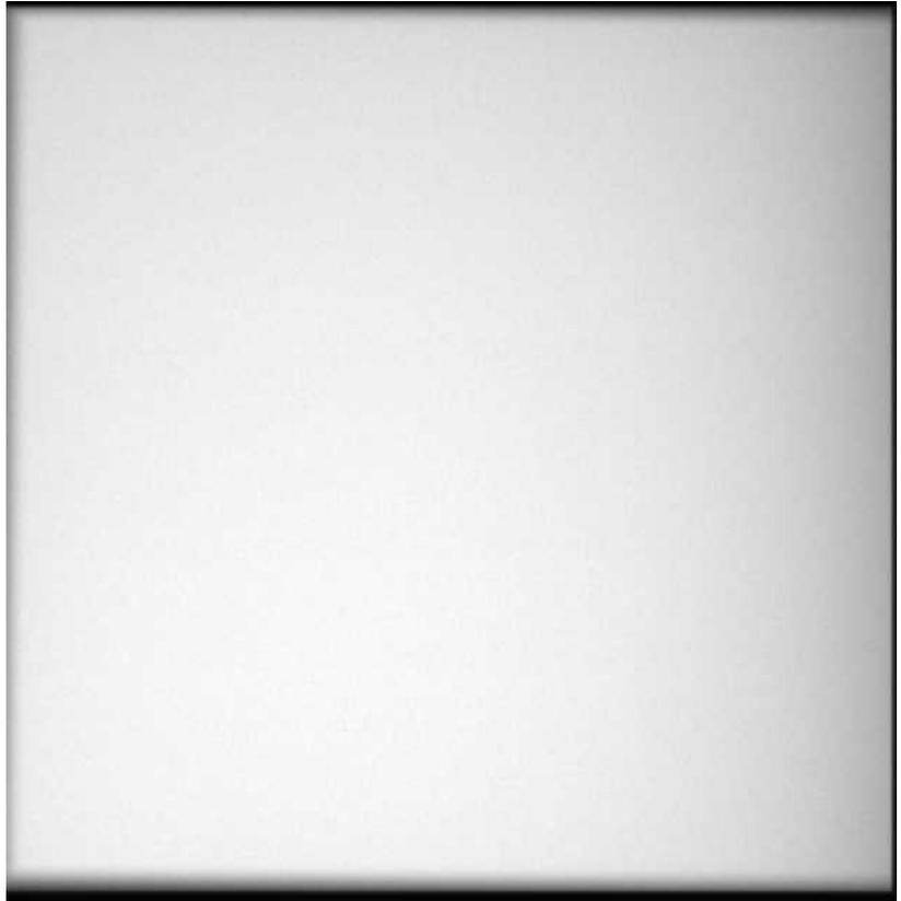
The diaphragm is correctly adjusted if a black surrounding edge can be detected.
