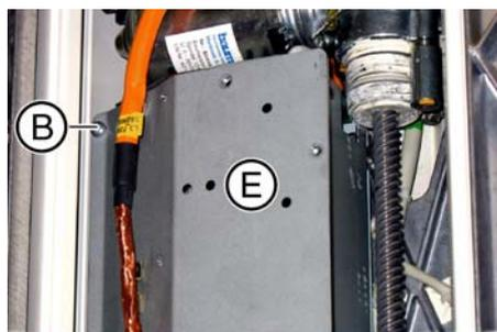
5. Loosen all the left-hand screws (B) of the protective plates (E).
