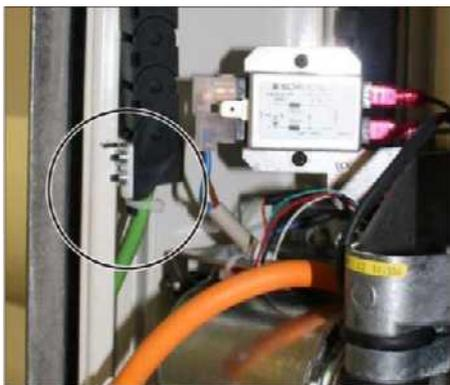
13. Unscrew the angle brackets on both sides of the cable track.
