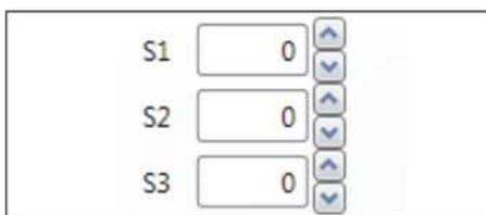
6. If adjustment is OK (the adjustment values in the text boxes are equal to zero), save the values. [ → 197]
