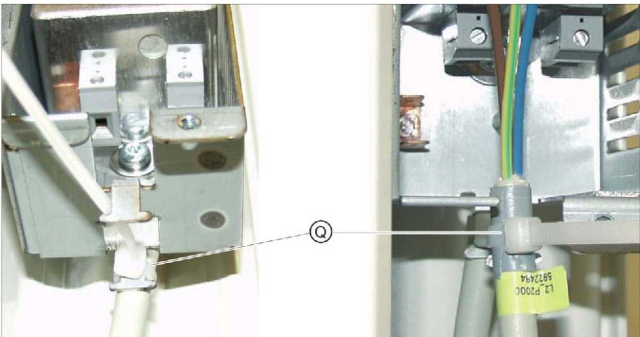
3. Attach cable **L2** first to the lower strain relief (photo on the left) and then to the upper strain relief (photo on the right) (**Q**) of board **DX32**.
