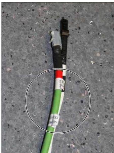
20. Fasten the two (new) cables together with adhesive tape above the flag labels.
