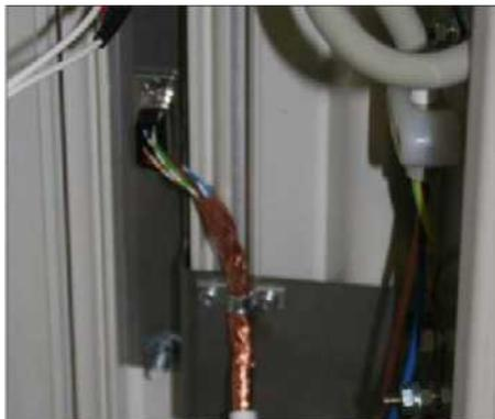
15. With defective cable **L117**: Unscrew cable **L117** from the interface board and remove the shield.
