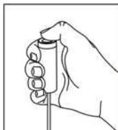
4. Press the release button. Press and hold down the button until the exposure is complete, the preview image is displayed in the exposure window, and the acoustic signal that indicates the end of the exposure (double beep) sounds (if it has been configured).
