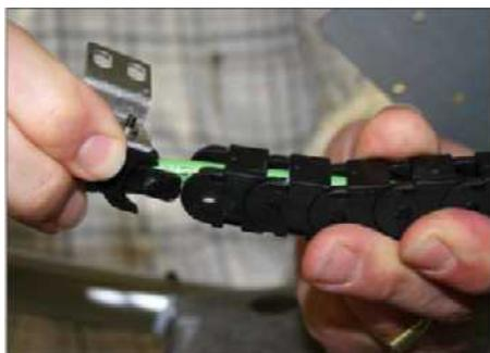
14. Remove the motor-side end piece from the cable track.
