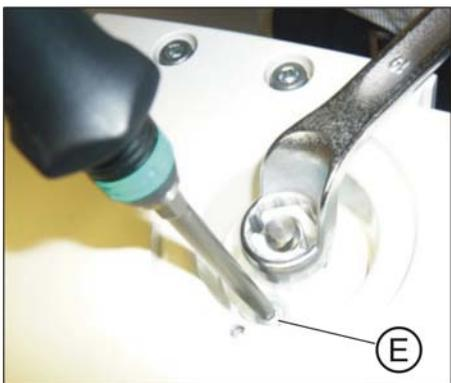
3. Attach the socket wrench (SW19) to the spindle. Hold it firmly in place while you unscrew the 2nd of the two screws (E).
