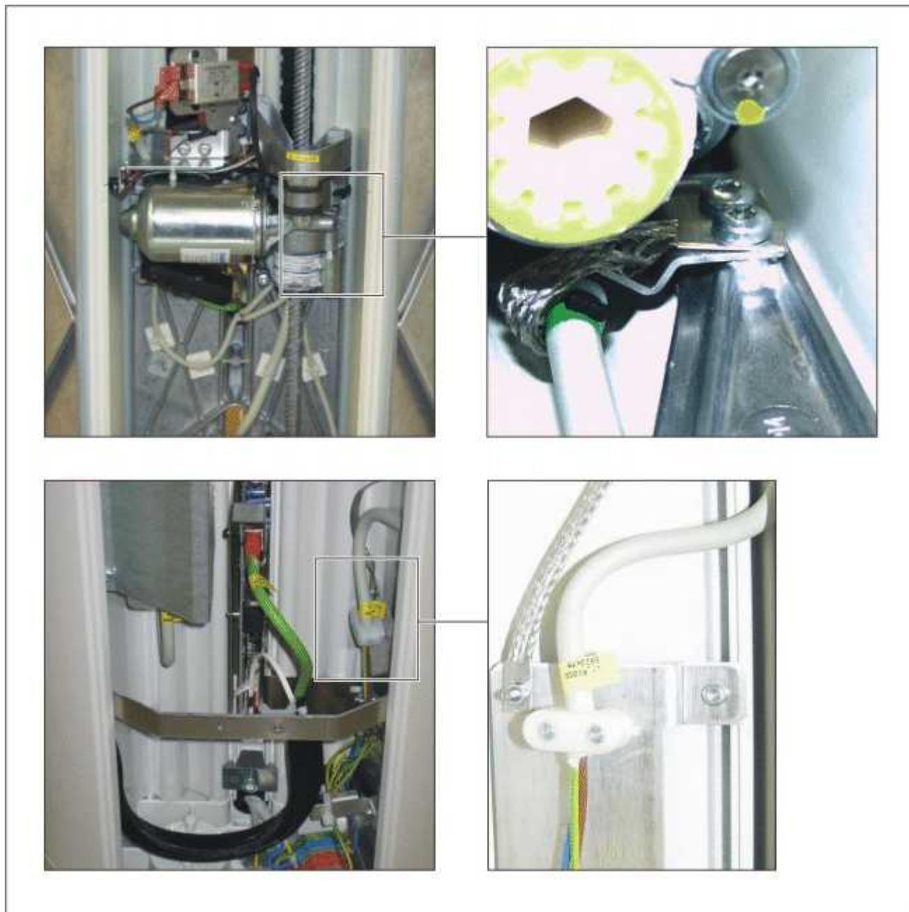
**Check whether the grounding straps have complete and firm contact**
