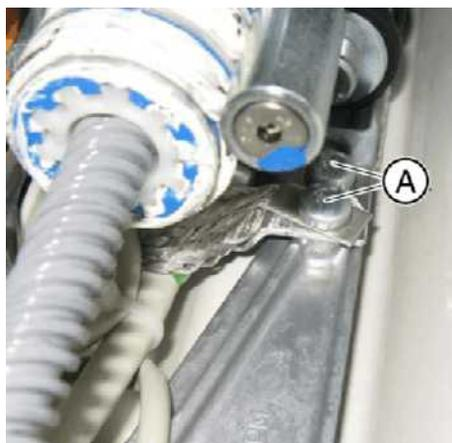
3. Loosen the two screws (A).
