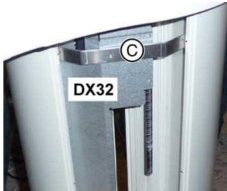
1. Unscrew the bracket (C). The bracket (C) is located in front of board DX32.
