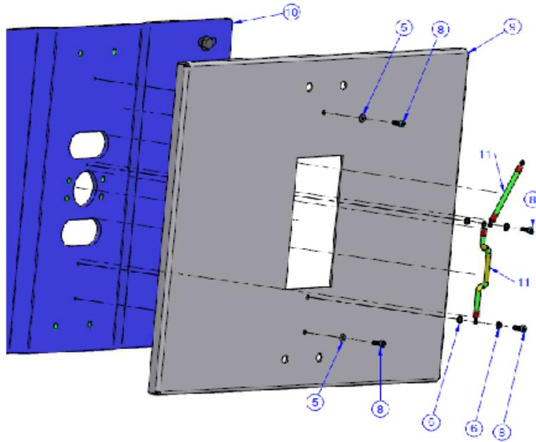
8. Fix the control unit on the cover with 6 screws M8x16(8) and 6 washers M8(7).
