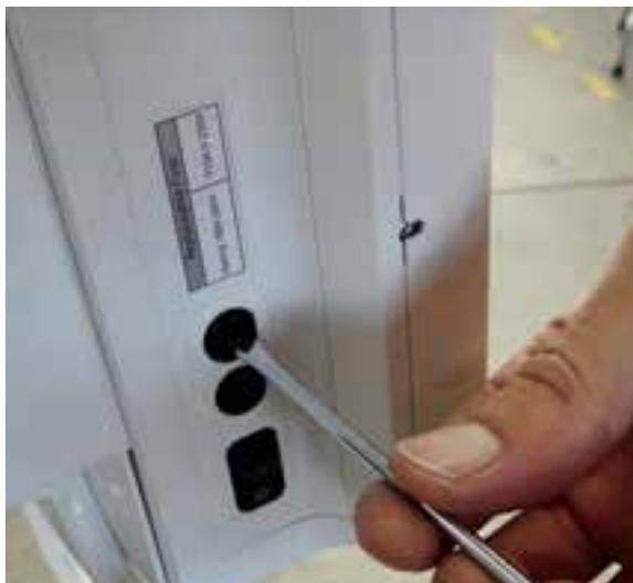
Unscrew half turn counter-clockwise with flat screwdriver the fuse holder F2
