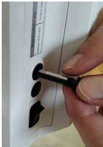
Screw half turn clockwise with flat screwdriver the fuse holder
