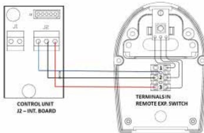
4. Arrange connections in the remote exposure switch as shown below, use the cable ties provided to fix the cable and always respect polarity.
