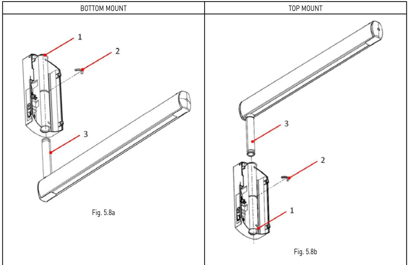
The bracket is provided from the factory with a ground cable already installed in the bracket, ready to be connected. During the operation of insertion of the bracket tube in the wall plate hole, it is suggested first to insert the cable in the tube pushing it gently inside, then fix the bracket by the half moon clip, take the ground cable out from the holes (X) of the wall plate and then fix it properly to the dedicated ground point prepared in the wall plate.
