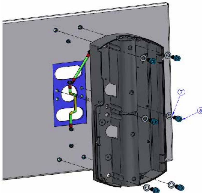
9. Fix the ground wire(11) with 1 screw M4x10(9) and double milled washers(6).
