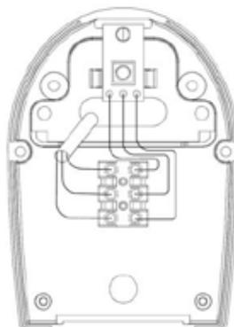
5. Close the front cover (4) then screw in the fixing screws (5).
