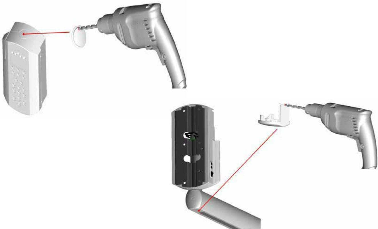
Cables routing change basing on installation types, please refer to images below for details:
