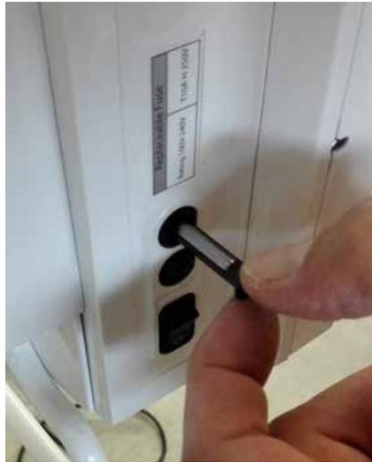
insert the fuse supplied WITH THE MOBILE STAND KIT in the fuse holder
