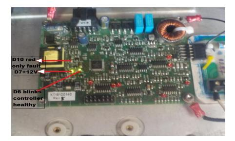
Console Extension PCB-INTERNAL (301-000340-0) Indication details.
