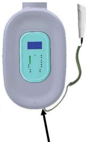
Figure 43: Fix exposure switch cable
