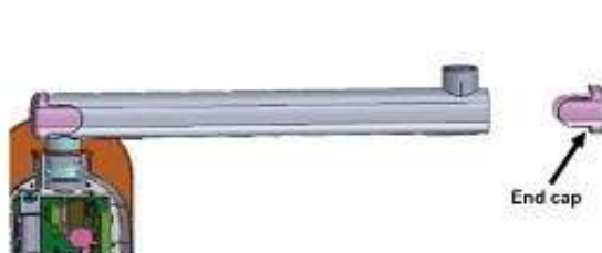
Figure 26: Remove end cap (M3x6 self tapping Counter sunk screws )Use screw driver
