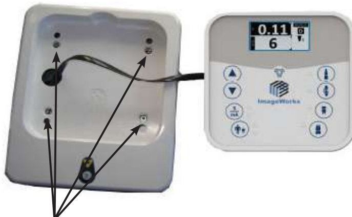
Figure 38-: 4 M3x6Hex socket head cap screws
