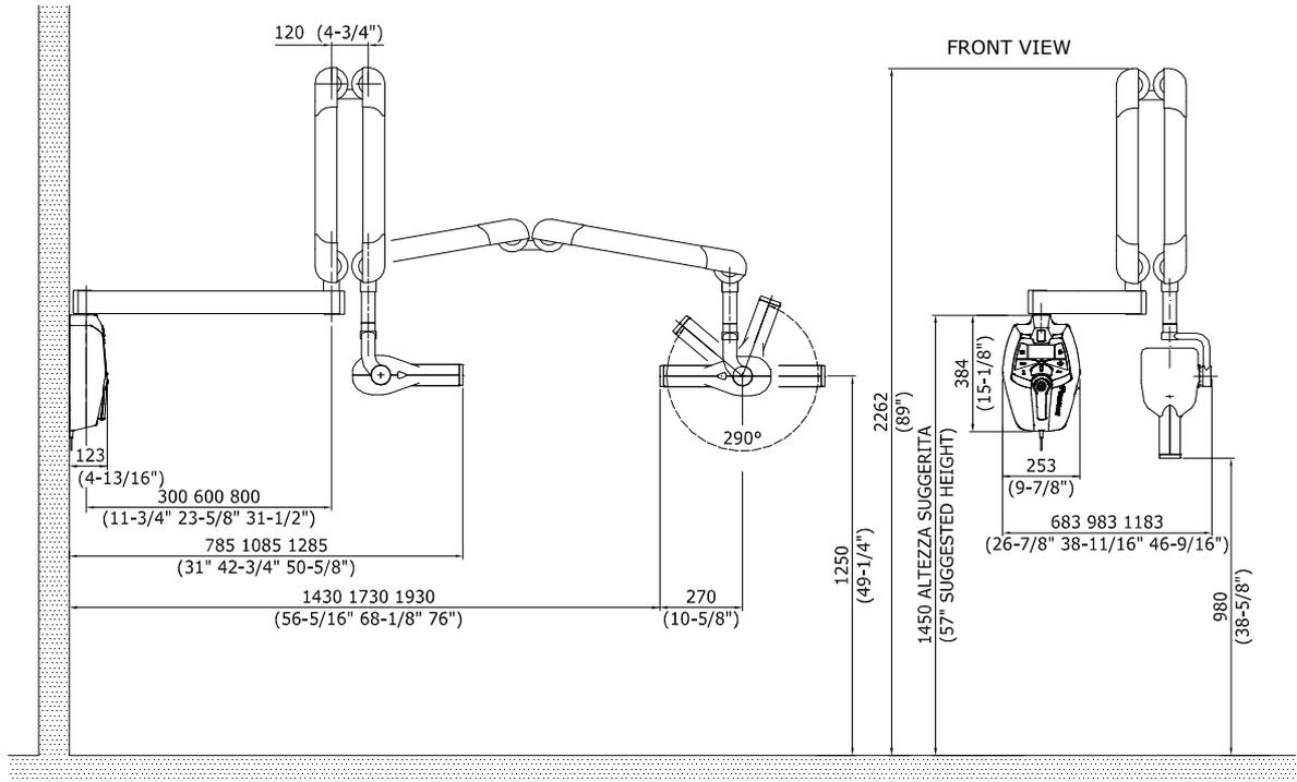
Figure 4-1: Dimensions of the wall version
