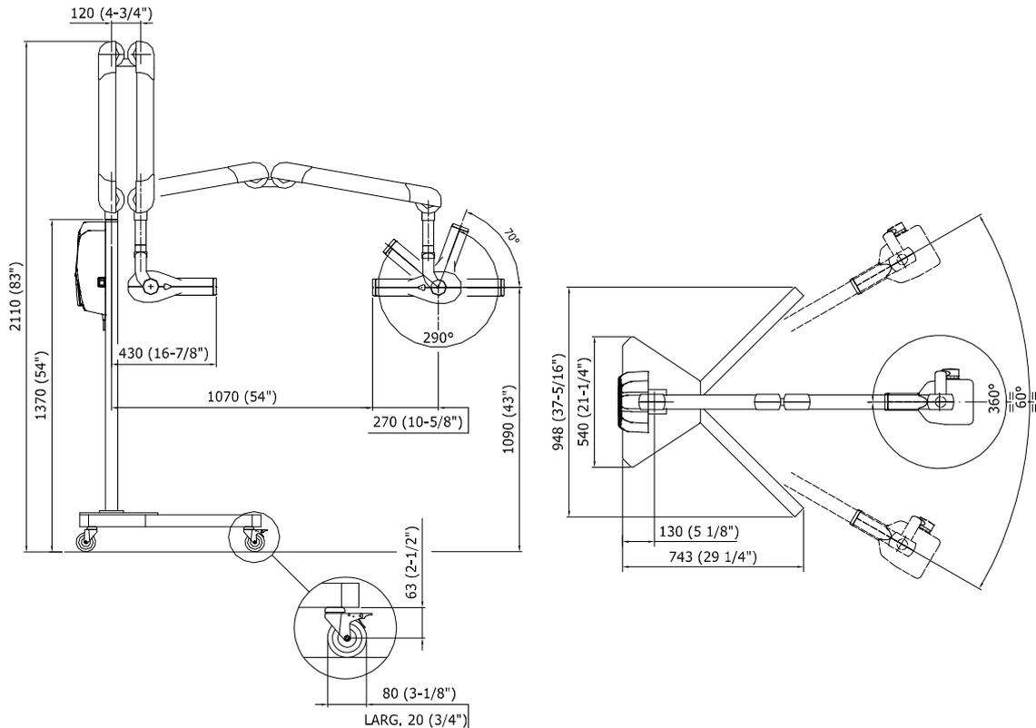
Figure 4-2: Dimensions of the mobile stand version
