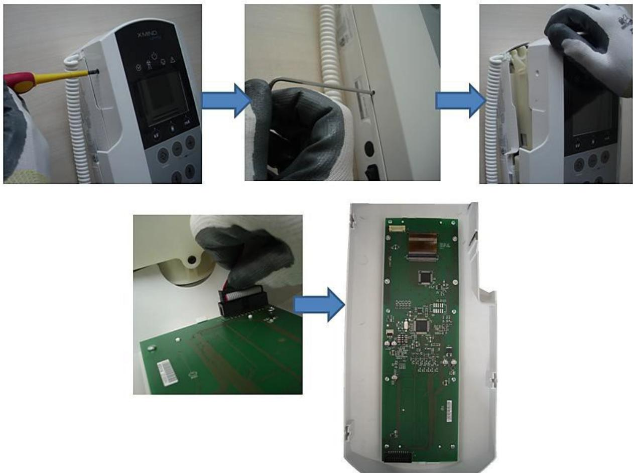
Follow step by step the procedure shown above to dismount the RXCD board
