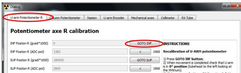
h. When movement is completed and U-arm is in the zero position (tubehead at the left looking at X-MIND trium from the front) click on arrow button of INF position field.
