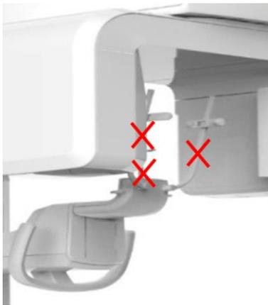
h. **Only for CEPH models:** place CEPH craniostat in AP position, rotate CEPH nasion in horizontal position and open at their maximum the ear rests.
