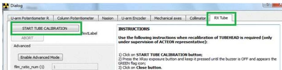
h. Keep continuously pressed the X-ray exposure button
